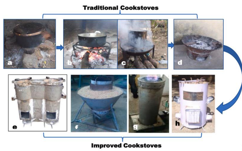
Figure 1: (a) Three-stone open fire, (b and c) Metallic open fire, (d) Traditional charcoal stove, (e) Natural-draft double burner biomass cookstove, (f) Husk biomass cookstove, (g) Inverted downdraft gasifier cookstove, (h) Improved biomass cookstove [22]
